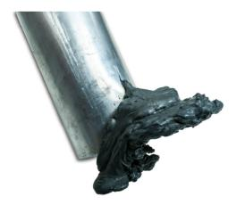
Most modern power capacitors are fitted with pressure release valves or complete pressure release caps, which enables the capacitor to alleviate the internal pressure should a failure occur.
