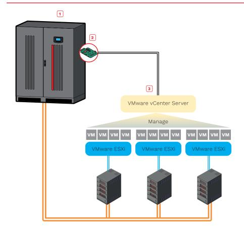
NetMan 208 should be used for managing Esxi hosts and vCenter servers, enabling you to manage your virtual network to perform shutdown or live migrations of active virtual machines as well as shutdown of physical hosts with delay and priority.
