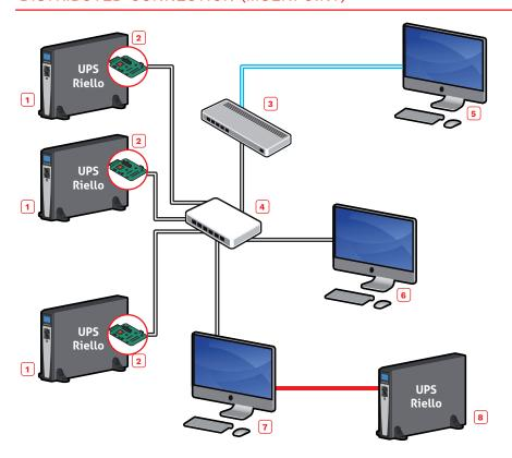
Connection with more than 1 UPS. The FULL version of PowerShield<sup>3</sup> software is required as well as a NetMan 208 communication board on each UPS.
