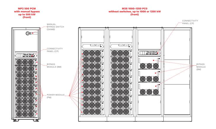
with input, bypass, output and manual bypass switches up to 1000 or 1250 kW CONNECTIVITY PANEL (CP) OUTPUT SWITCH (SWOUT) **-**MANUAL BYPASS INPUT SWITCH SWITCH (SWMB) (SWIN) BYPASS SWITCH (SWBYP) POWER MODULE (PM) .. BYPASS MODULE (BM)
