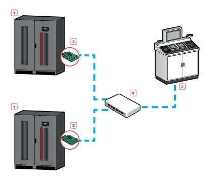
For UPS management in industrial or civil environments requiring Modbus protocol communication over Ethernet.
